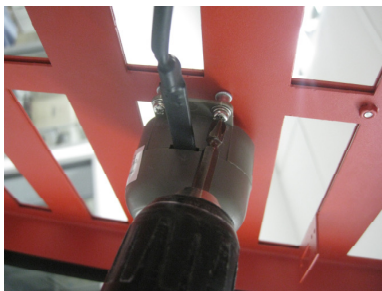
Figure 5.10. Remove doughnut sensor housing
