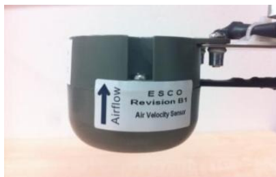
Figure 5.11. Airflow sensor direction
