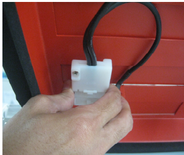
Figure 5.8. Disconnecting Airflow sensor Cable
