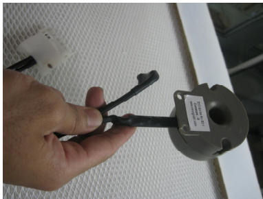
Figure 5.9. Remove Temperature sensor
