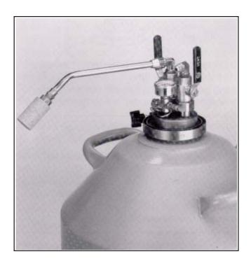
Vent all pressure from a Dewar before attempting to remove the Liquid Withdrawal Device. If the band clamp securing the LWD to a dewar is loosened while there is pressure in the Dewar, cold gas or liquid could be expelled causing personal injury.
